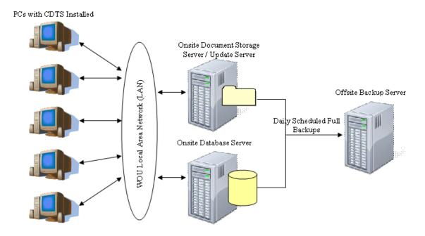
Figure 3: CDTS system architecture
