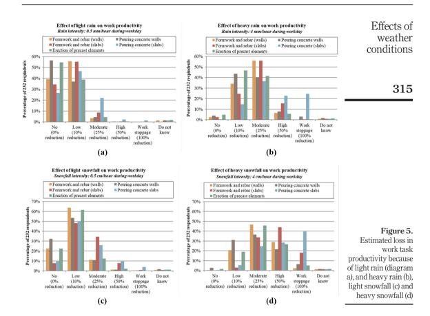
performed on horizontal areas (e.g. formwork and rebar, and pouring of slabs) are more sensitive to heavy rain compared with work tasks performed on vertical surfaces (concrete walls).
