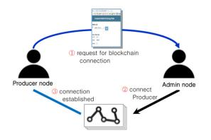
Figure 1. Process of connecting producer node to blockchain
