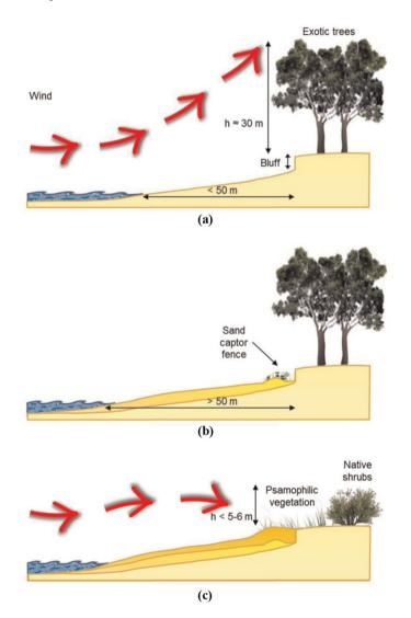
Figure 5. Schematic representation of the beach profile before (a) and after (b) the soft intervention in 2013 (inspired by Kim *et al.*, 2014); the desired near-future state (c) shows an ideal rebuilding of both beach profile
