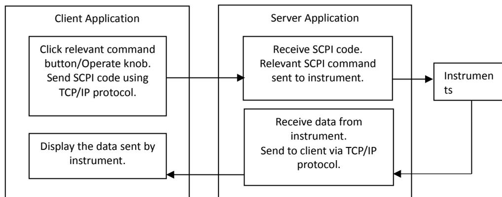
**Figure 2** Instrument control architecture of the ORL system
