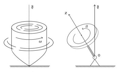
**Figure 2.** Generation of a gyroscope's external torque
