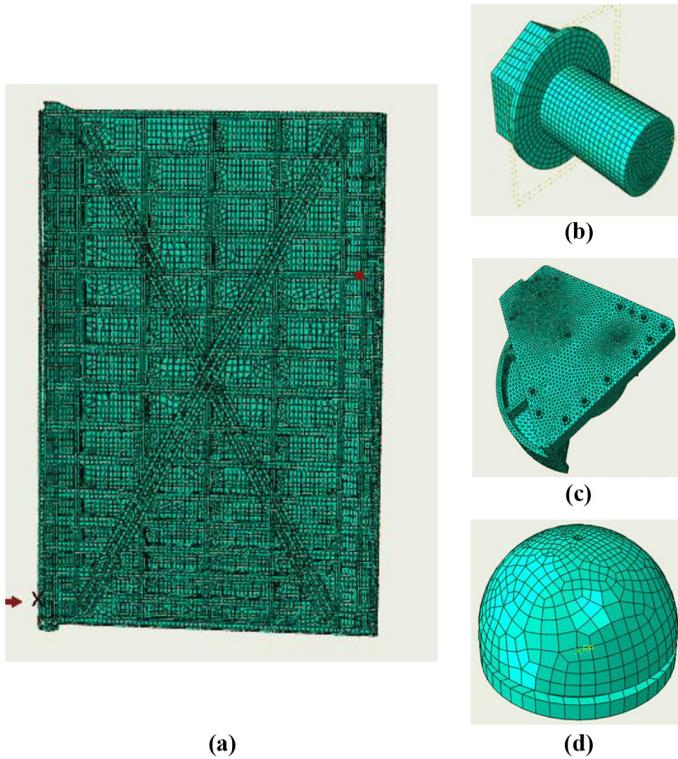
**Figure 2.** (a) Mesh for the 3D shell elements of the gate; (b) and (c) mesh of the 3D solid continuous elements in the bolts and pintle socket; and (d) mesh of the rigid elements in the pintle ball
