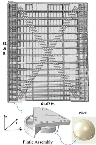
**Figure 1.** Leaf dimensions of a downstream view of the 3D numerical model in Abaqus
