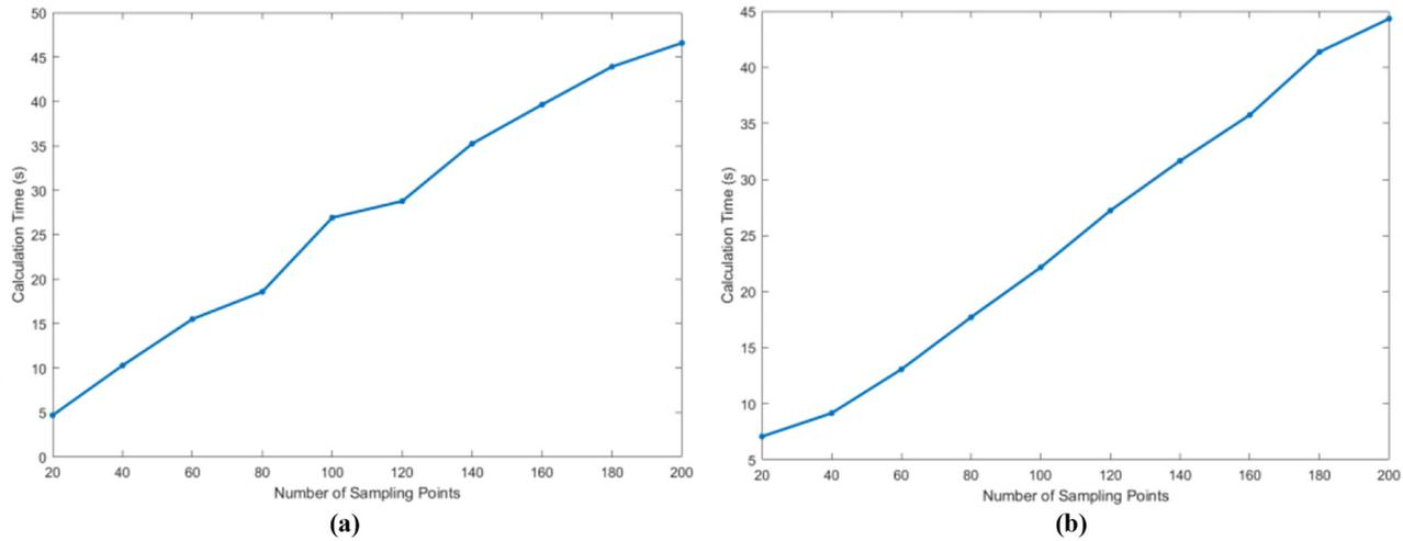
**Notes:** (a) Calculation time of numerical method for S-bends path; (b) calculation time of numerical method for helix path
