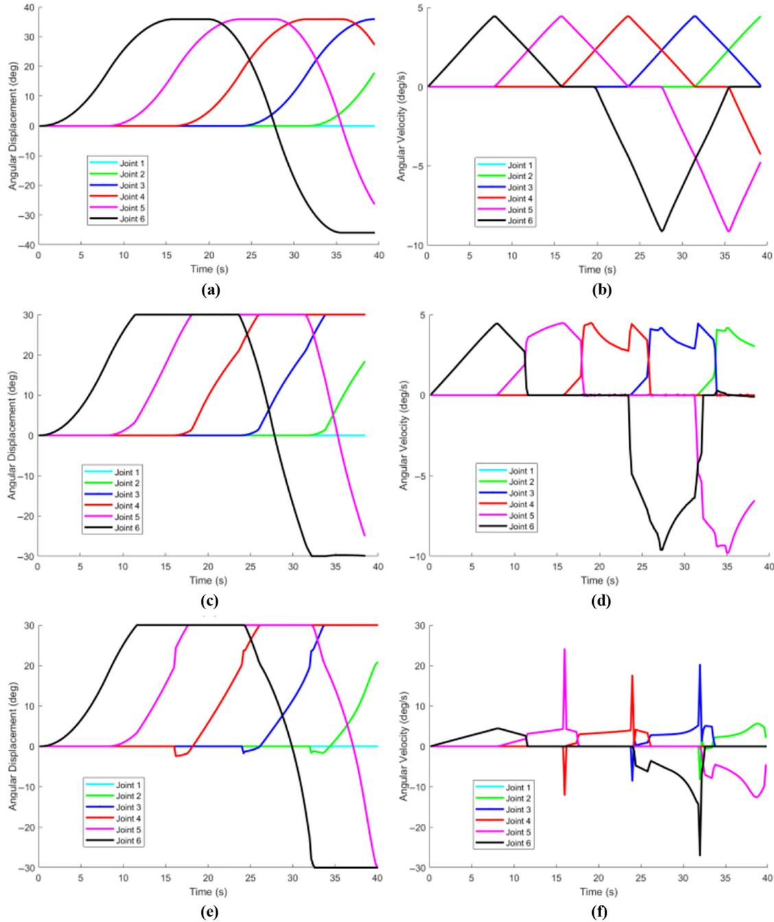
**Notes:** (a) Angular displacement of path-following method without joint limits; (b) angular velocity of path-following method without joint limits; (c) angular displacement of path-following method with joint limits; (d) angular velocity of path-following method with joint limits; (e) angular displacement of numerical path-following method; (f) angular velocity of numerical path-following method
