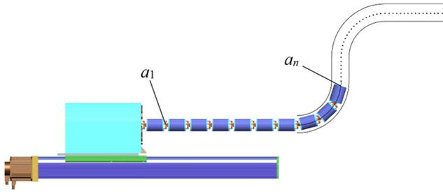
points, the key of path-following method is that the distance between the joint points of the manipulator and the targets point of the path curve should be kept minimum for each step. Thus, the problem turns into how to find each joint point closest to the target points quickly in turn.
