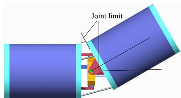
Figure 7 Incorporating joint constraints within path-following method
