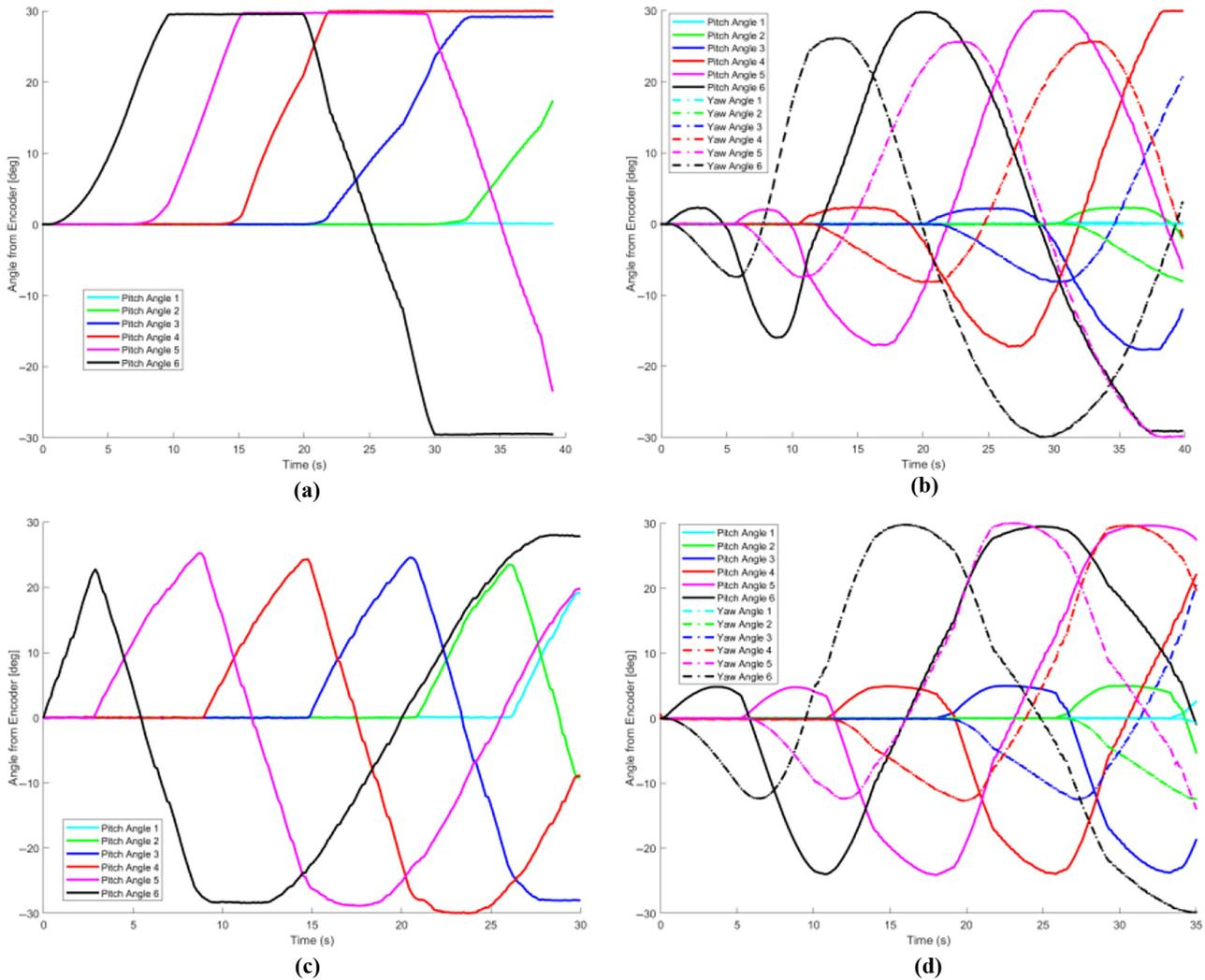
Notes: (a) The bending angles of joints in S-bends path; (b) the bending angles of joints in helix path; (c) the bending angles of joints in sinusoidal path; (d) the bending angles of joints in helix path
