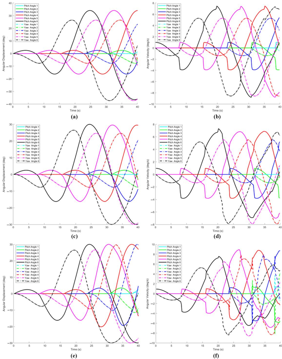
**Notes:** (a) Angular displacement of path-following method without joint limits; (b) angular velocity of path-following method without joint limits; (c) angular displacement of path following method with joint limits; (d) angular velocity of path following method with joint limits; (e) angular displacement of numerical path-following method; (f) angular velocity of numerical path-following method
