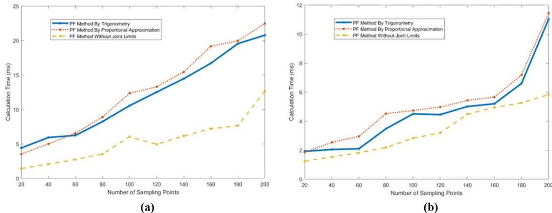
Notes: (a) Calculation time of path-following methods for S-bends path; (b) calculation time of path-following methods for helix path
