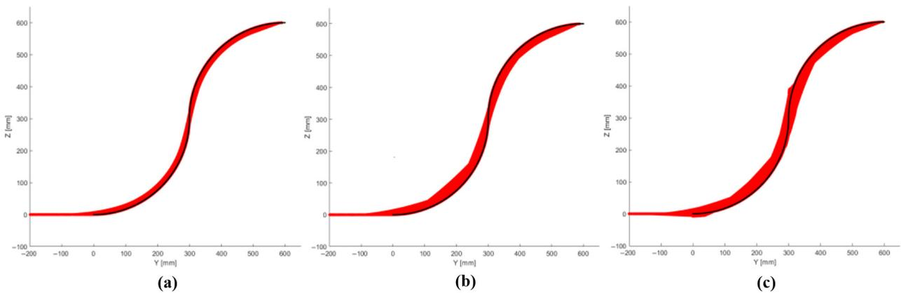
**Notes:** (a) Envelop of path-following method without joint limits; (b) envelope of pathfollowing method with joint limits; (c) envelope of numerical method
