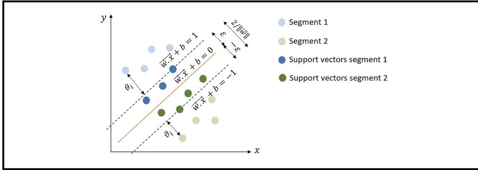
fitting function  $f(\vec{x}) = \vec{w} \cdot \vec{x} + b$  by minimizing the regularized risk function  $(1/2)\|\vec{w}\|^2 + C \sum_{i=1}^N (\theta_i + \vartheta_i)$ , where  $C$  is the regularization parameter,  $\theta_i$  and  $\vartheta_i$  are distances from actual value  $y_i$  to the boundary values of  $\varepsilon$ . Thus, the nonlinear mapping function  $f(\vec{x})$  can be generated by applying the Lagrange multiplier (Yao *et al.*, 2021),
