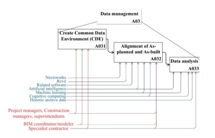
Figure 6. Data management process at the as-built generation stage
